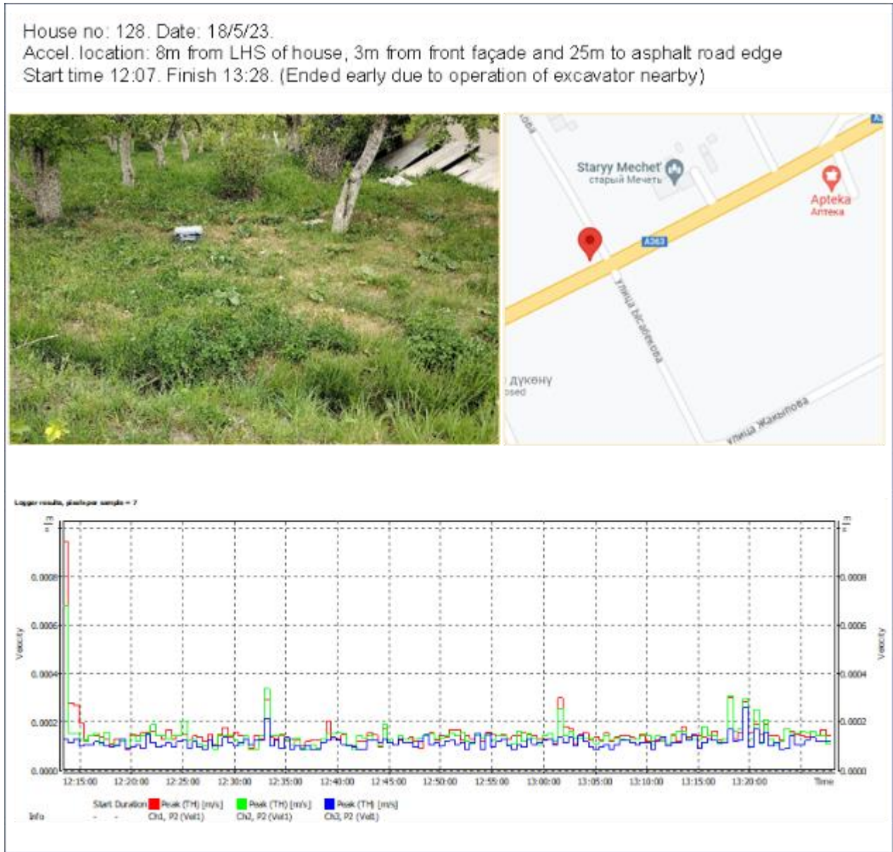
Figure 49: Vibration monitoring at Location L3: Darkan
